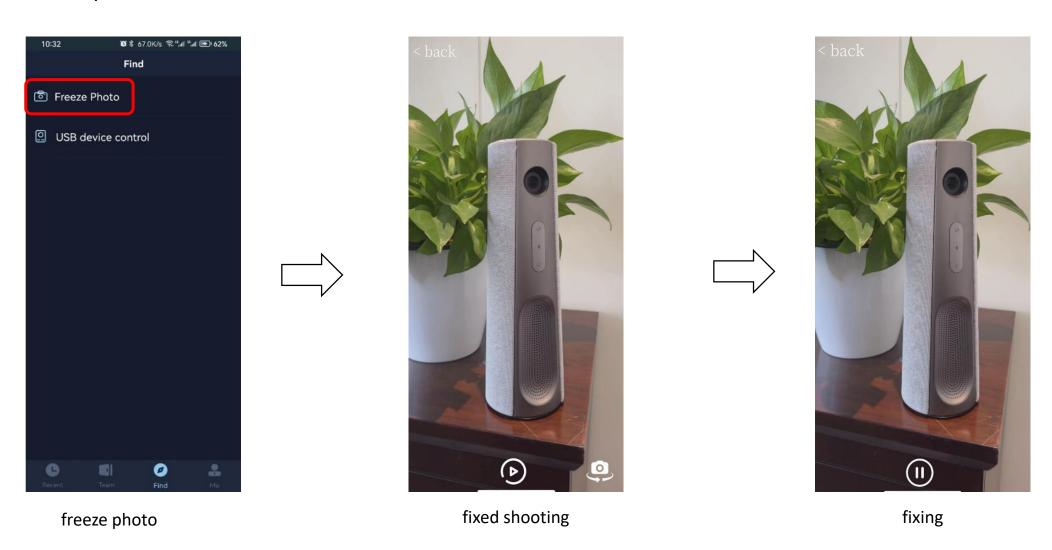
Note: freeze photo is used with the mobile phone screen function with the Teamfree device. After the fixed shoot. The camera will keep the image in the fixed freeze, you can observe the shooting details
