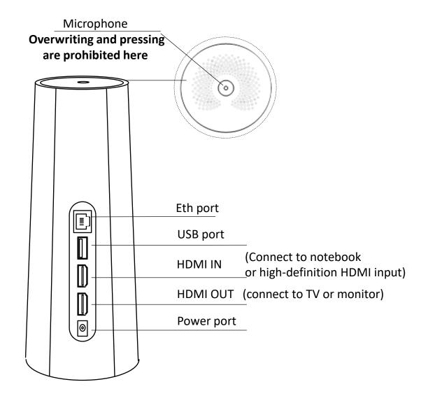
Note: The device has no power switch. It will turn on when connected to a power source and shuts down after disconnection
